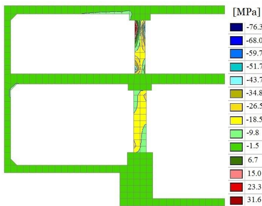
Figure 8. Distribution of vertical normal stresses (MPa) in a model fragment (half of the vestibule structure) at an impulse value of I_1=2000 \text{ kg}\cdot\text{m/s}
