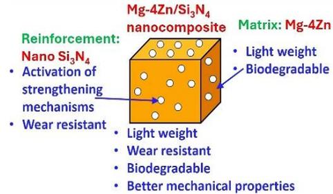
Figure 2. Using Si<sub>3</sub>N<sub>4</sub> nanoparticles to improve wear properties of Mg-4Zn alloy
