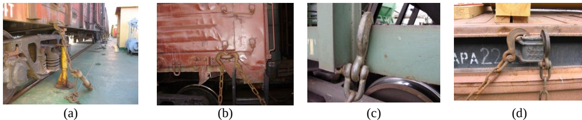
Figure 1. Figure caption Randomness of the places of fastening of chain ties to the structural elements of wagons: a) a covered wagon on the ferry "Heroi Shipki"; b) an open wagon on the ferry "Greifswald"; c) a hopper wagon on the ferry "Petrovsk"; d) a flat wagon on the ferry "Heroi Odessa"
