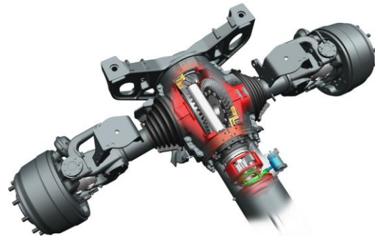
Figure 3. Independently suspended wheels [32]
