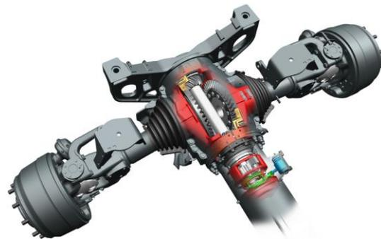
Figure 3. Independently suspended wheels [32]
