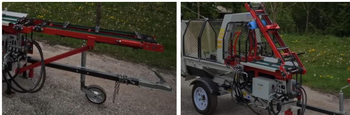
Figure 11. A real implementation of the designed chain driven conveyor in a working position (left) and in a transport position (right)
