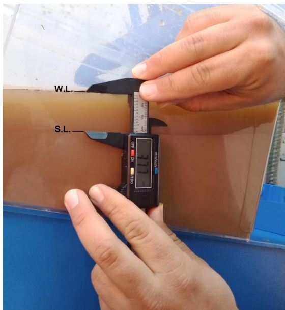
Figure 8. A photo of controlling the horizontalization of the liquefied SLM test specimens
