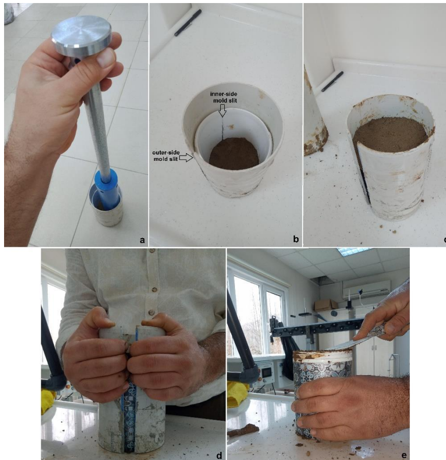
Figure 4. Specimen molding for the HS test: a) soil layer compaction, b) double molds with slits, c) soil specimen level exceeded the height of the inner-side mold, d) opening the outer side mold's slit, e) removing the soil above the inner-side mold by using spatula
