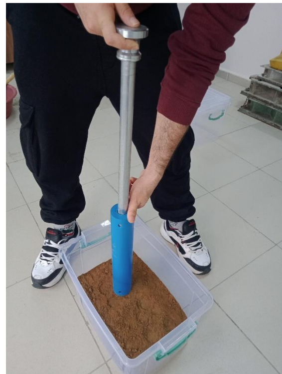
Figure 6. A photo from the soil layer compaction work for the SLM test specimen preparation
