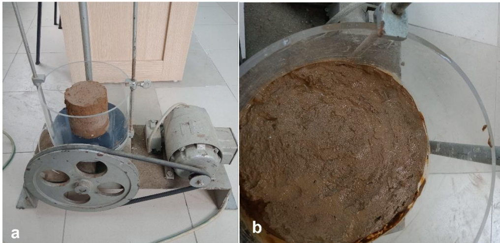
Figure 5. HS (Horizontal shaking) test mechanism and a specimen before the load cycles (a), liquefaction after the load cycles (b)
