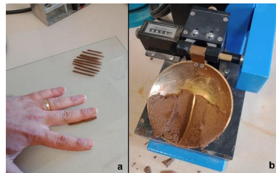
Figure 3. The plastic (a) and liquid limit (b) tests
