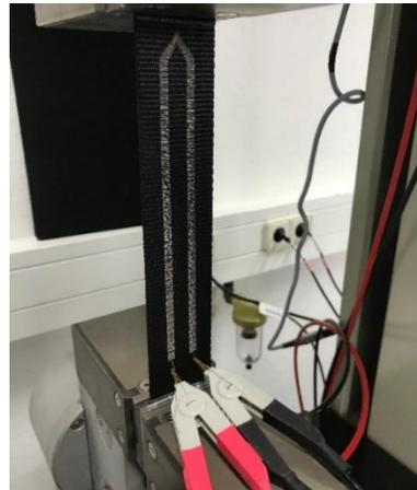
Figure 14. Loose stitch ends contacted with crocodile clamps
