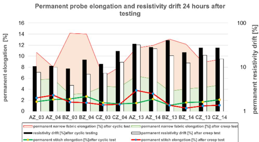
Figure 26. Probe permanent elongation and resistivity creep 24 hours after testing procedure
