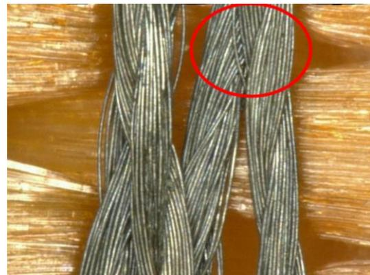
**Figure 1.** Overlapping conductive yarn loops
