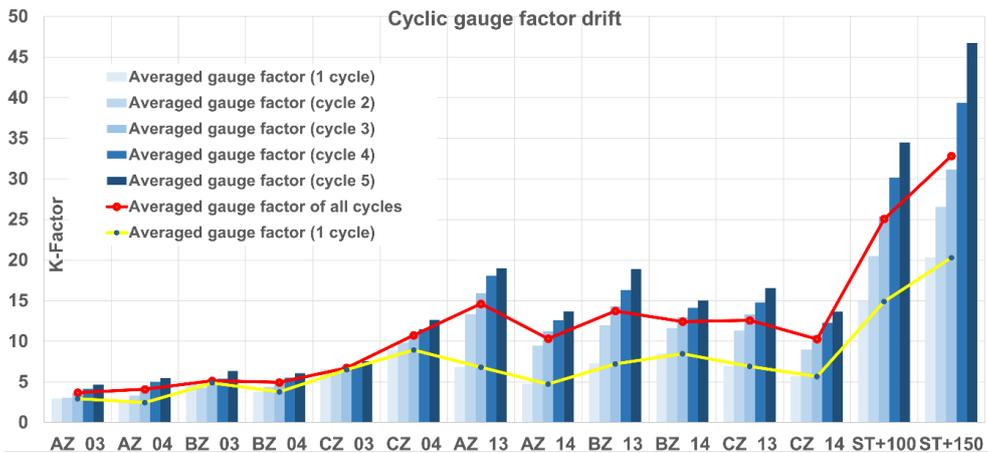
Figure 21. Probe cyclic strain gauge factor drift
