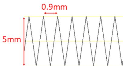
**Figure 8.** Stitch properties ZigZag\_V2\_Axial
