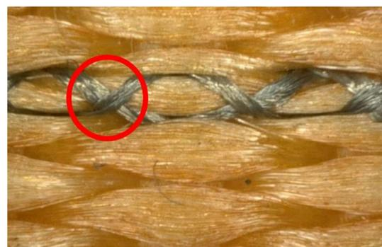
**Figure 2.** Cross sectioning conductive yarn loops
