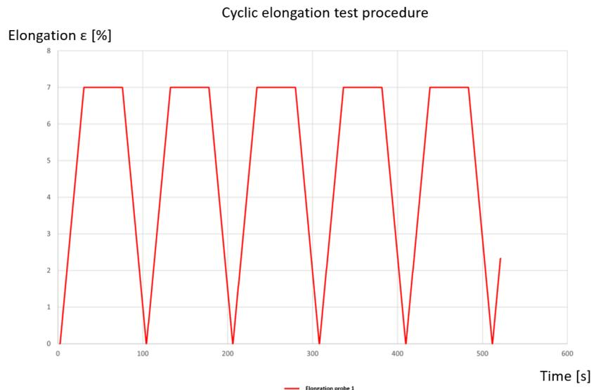
Figure 15. Cyclic elongation test routine
