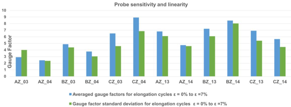
Figure 17. Probe averaged gauge factors (blue) and gauge factor linear deviation (green)
