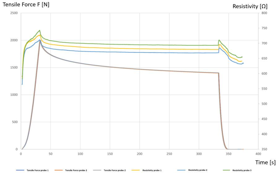
Figure 24. Probe C\_Z0\_3 resistivity creep compared with strain force creep
