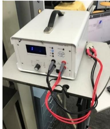
Figure 13. Elabo R-Meter/SRM 05
