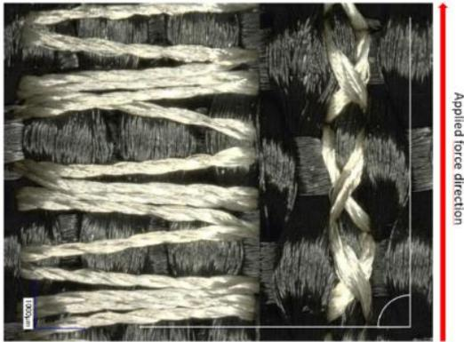
**Figure 22.** ZigZag\_V2\_Axial (left) and ZigZag\_Double\_V2 (right) loop orientation in applied force direction.
