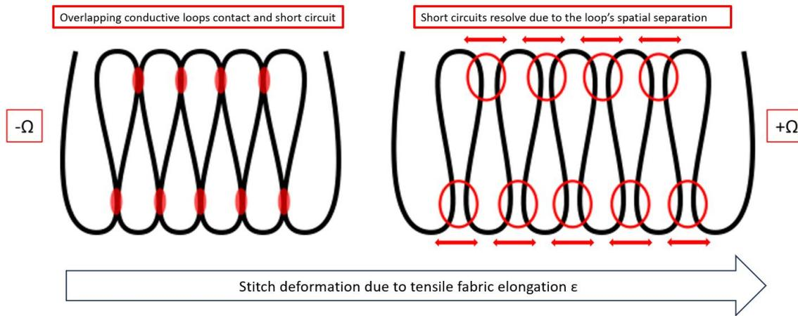
Figure 3. Schematic representation of the mechanism of increasing resistance by dissolving the yarn contacting
