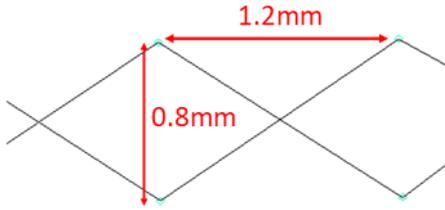
Figure 10. Stitch properties ZigZag\_Double\_V2
