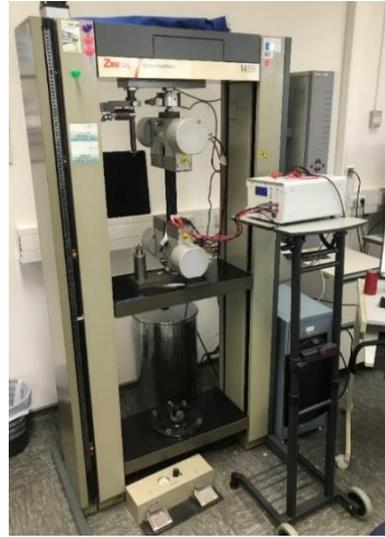
Figure 12. Zwick 1455 20kN tensile testing machine
