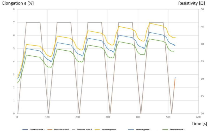
Figure 19. Probe C\_Z0\_3 resistivity drift over multiple cycles
