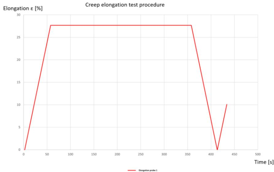
Figure 16. Creep elongation test routine
