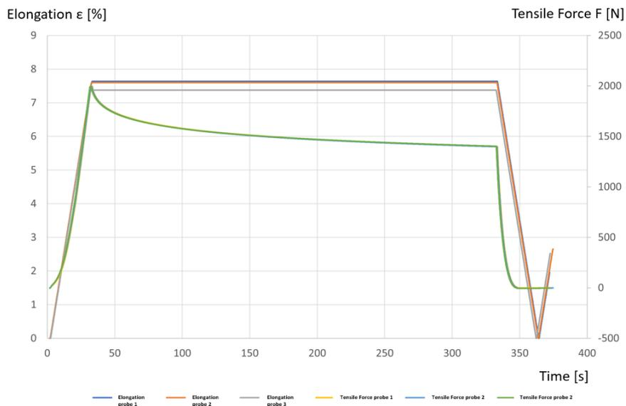
**Figure 23.** Probe C\_Z0\_3 regressive strain force creep
