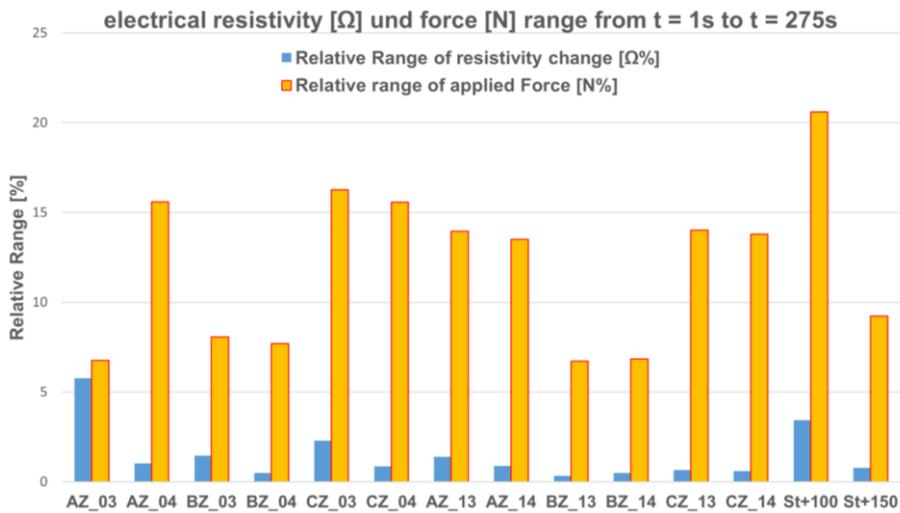
Figure 25. Probe resistivity and strain force creep behaviour
