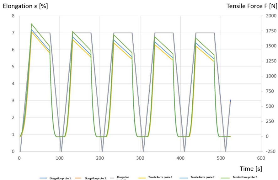
Figure 18. Probe C\_Z0\_3 strain force drifting over multiple elongation cycles
