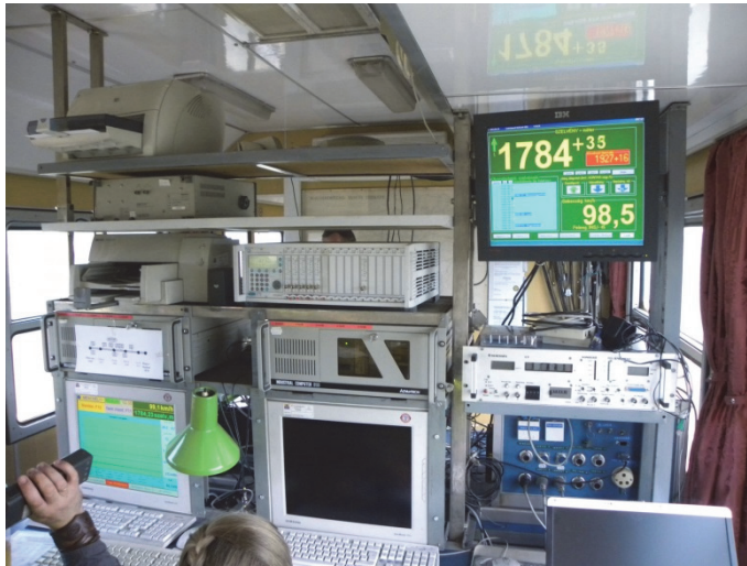
Figure 3. Several parameters on the display of VMK–002 traction measuring car
